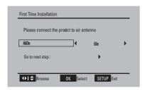
4 Select the antenna type as [Air], then press ▼ to select [Go to next step:] and press OK to confirm.
